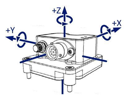
Where possible the CSG should be mounted as close to the centre of gravity.
