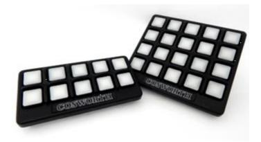
The RSP features user-configurable CAN allowing for IDs, rates of the packets as well as BUS termination. The state of each switch is transmitted over CAN at 200Hz by default as well as the additional 2 digital inputs providing external switches. All communication is made through a single double density Deutsch Autosport connector including the RS232 Debug comms.
