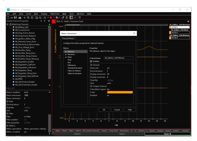
Metric Definition Extensions - Metrics can be used to generate output channels, which can then be consumed in the same way as all other channels. Extensions can be configured both for Basic Function Editor metrics, and script generated metrics. The Metrics tab can be found under Tools > Advanced Maths > Basic Function Editor.
