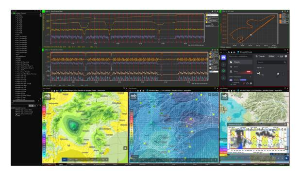
Recovery of real-time data – Toolbox 13 Advanced Real-time Options now allow real-time data to be configured and cached to disk. Data can be retained for a configurable number of hours, it is then possible to configure real-time outings to load any available cached data when reconnecting (following app closure), which also then enables all previous data to be viewed, and metrics to be calculated from that data. Cached Data is loaded automatically when the workbook is reopened.
