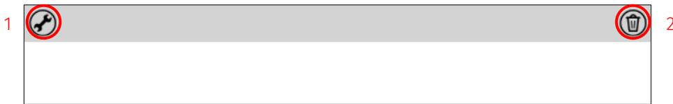
When the display setting menu is open you can import a track map (.pxt file format) (1). You can use the 'bin' tool to delete a track map (2).
