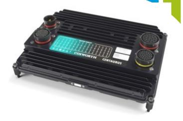
New for Cosworth's power box range is support for ethernet driven displays and steering wheels (CDU 4.3, 7, 10.3, CCW Mk2, CCW Mk3, and I/O expansion via EtherCAT™, providing market leading levels of synchronicity with the SJU (Synchronous Junction Unit).
