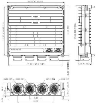
The Antares 8 is designed to function up to a maximum RPM of 16,000rpm when running GDI, or 22,000rpm when running with port fuelling only. There are four lambda sensor inputs, which will accept NTK/Bosch style wideband sensors. There are also eight specialised knock inputs with a software enabled gain stage.
