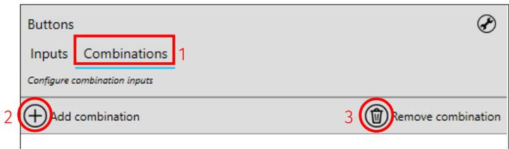
You can configure the new button combination. Name the combination (1), and then provide an optional description (2). You can select if the combination is enabled in the setup (3). You can then use the **Choose a Strategy** option to select the strategy condition (4/5).
