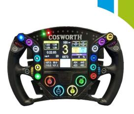
backlight independently for each button or rotary and brightness controlled in two zones - button backlight and rotary backlight.
