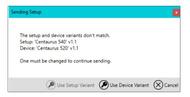
You can also change the setup variant on the main **Setups** page via the **Change Variant** option to avoid the 'Use Device Variant' prompt.
