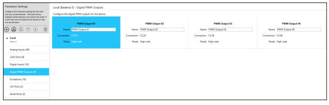
For devices with Digital PWM Output capability, you can configure the name of the Digital PWM Outputs on the **Hardware Settings** node (1.). Underneath each PWM Output label is a connection identifier in the format 'CX.Y', where X and Y are values that identify the connector and the pin of the device respectively (2). The PWM output **Mode** (high-side or low-side) is displayed (3).
