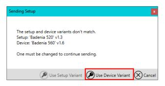
On the home page of the open setup, version information is displayed. If the device variant and setup variant do not match, a warning is displayed in the **Health Check** section.
